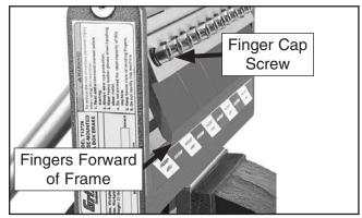
Figure 8. Fingers positioned forward of frame.
